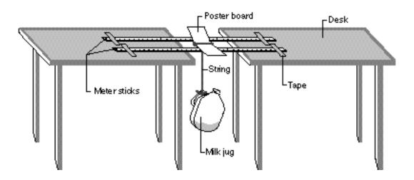
20. Record the data on the NASA Connect Activity Student Record Sheet (page 13). Calculate the flex strength using the formula.
