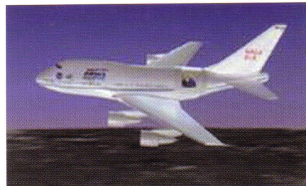
NASA's Stratospheric Observatory for Infrared Astronomy has a large infrared telescope on a modified Boeing 747
